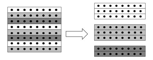
The usage of **Rowwise Cyclic-Striped Decomposition** allows to achieve best characteristics of calculation load balancing among the subtasks
