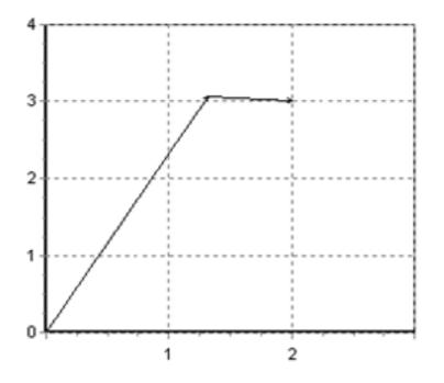
Iterations of the conjugate gradient method for solving the system of two linear equations:
